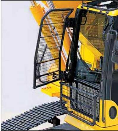
Cab front full height guard level 1 (ISO 10262)
