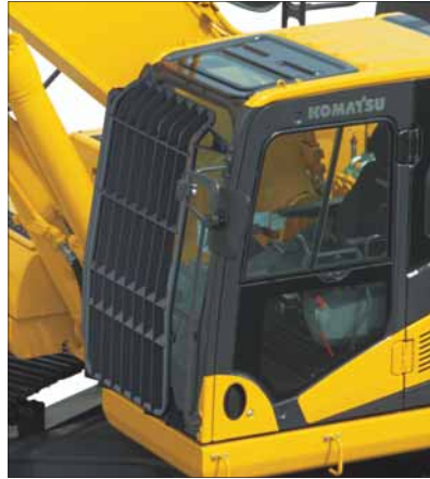
Cab front full height guard level 2 (ISO 10262)
